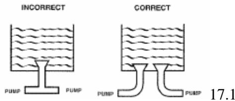
The in-flow should not cause interference with the drain pipe (Figure 17-2).
