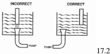
Drain pipe design must respect proper submergence (Figure 17-3). The submergence laws appear later.
